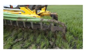
The Aerway tool bar will perforate the ground leaving 6" to 8" pockets that the effluent or manure slurry will fall into. There are two types of slurry deliveries: 1) broadcast prior to and after the rotary wheels perforate the ground, 2) direct deposit of the slurry behind each rotary wheel after it perforates the ground.
