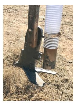
The most popular sweep is the Dietrich Sweep which is a hardened steel sweep designed for three different application rates. The ones LPD uses is the high flow model which will accommodate application rates between 10,000 and 40,00 GPA. Higher application rates will leave slurry on top of the ground.
