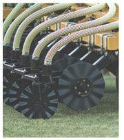
This type of tool bar uses a wavy or straight coulter to sweep the crop debris away from the path of injection.
