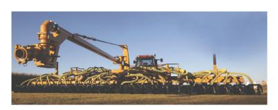
The resulting field does have some ridging or humps but not as bad as a sweep. The width of the tool bar and the fact it does not have to be removed from the ground on turn arounds makes it a popular choice for some situations.
