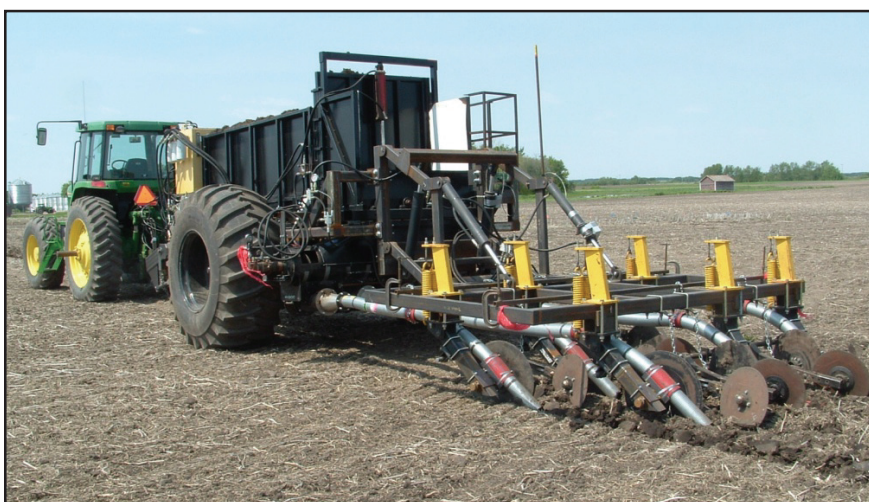
Figure 3. Solid-manure injection system (Hubert Landry, Prairie Agricultural Machinery Institute, PAMI)
