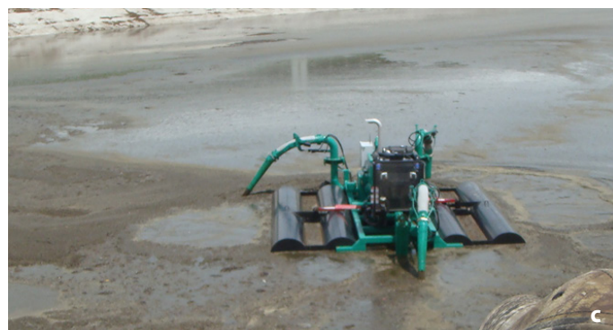
Figure 2. Types of agitators: a) pump, b) propeller (source: Dan Bolinger, Michigan State University), and c) boat (source: Kevin Erb, University of Wisconsin-Extension).
