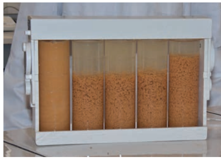
Figure 3. A jar test is used to determine the best polymer to treat sediment samples collected from a project's site.
