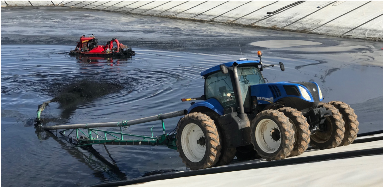
Agitation boat force feeder pumping an 80-million-gallon lagoon
